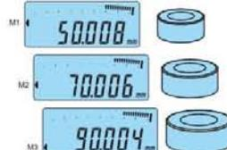
Up to 3 sets of reference values can be preset, including top/bottom tolerance limits.
