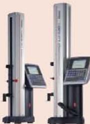
**Height Gauges with Data Processing Unit**
