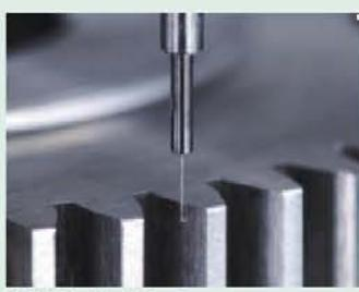
MPP-NANO Module 0.8 master gear measurement
