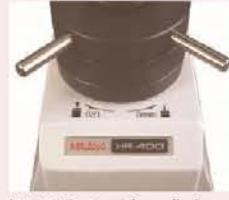
**HR-400** Automatic preliminary test force brake
