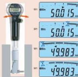
The ABSOLUTE Digimatic Bore Gauge detects the minimum value (true diameter) and holds it automatically.
