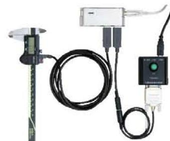
Sample application with USB Input Tool Direct
