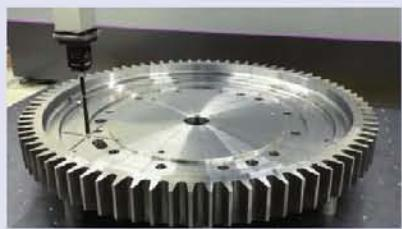
Scanning with probe SP80 and 100 mm stylus.
