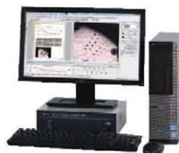
AVPAK-20 software 11AAC666 for automatic hardness testing systems. Software that supports control, testing and report creation related to hardness testing. Supports parameter setting and automatic measurement.
