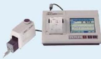
**Surface Roughness Measuring Instruments**
