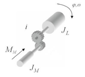
For the acceleration  $\alpha$  as a function depending on the ratio *i* in the drive train, the following applies:
