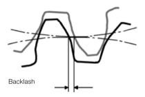
Torsional backlash is measured with the input shaft locked.
