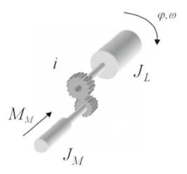
The following examination of the energy efficiency now also includes the ratio between the external mass moment of inertia and the mass moment of inertia of the motor. For this purpose, the external mass moment of inertia and the mass moment of the motor must first be converted with respect to a reference coordinate. The figure below shows the possible approaches
