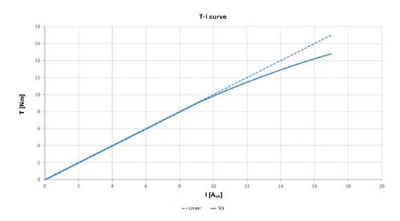
Here, it becomes clear that, starting at a motor current of 14  $A_{eff}$  the saturation already leads to a 10 % deviation to the proportional torque / current characteristic. The torque constant usually taken as a variable  $K_{\tau}$  is therefore reduced by half within the usable current range through the saturation
