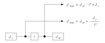
The coupling factor  $\lambda$  describes the ratio of the external mass moments of inertia to the mass moment of inertia of the drive. In this example, the reference coordinate is defined as the motor shaft. In accordance with the equation, the following applies to the coupling factor  $\lambda$ :
