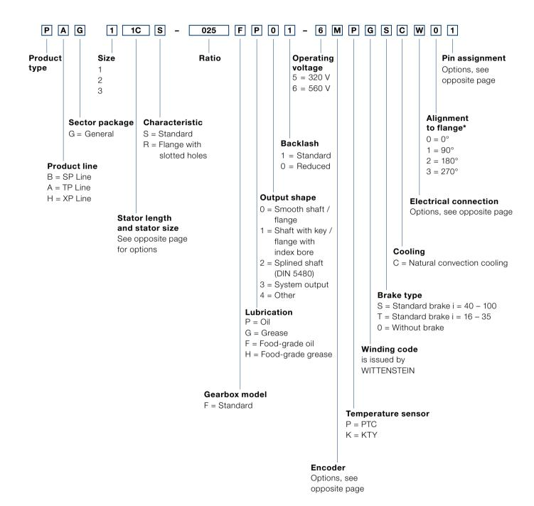
\* The position of the electrical connection with respect to the flange is relevant for XP Line with characteristic R (flange with slotted holes). This information relates to the offset of the integral sockets to the slotted holes as seen on the servo actuator from the rear.
